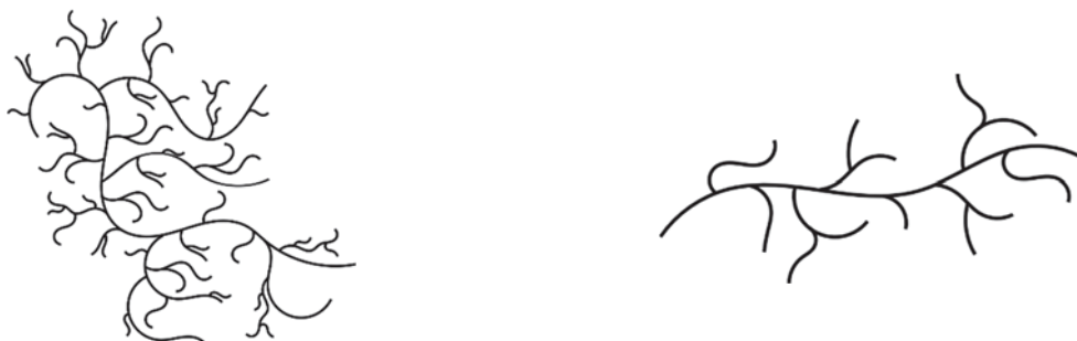
Fig. 2.: The microstructure of LDPE produced in autoclaves (left) and tubular reactors (right). Due to the back-mixing behavior of an autoclave, its product is tree-like branched. Tubular products are comb-like branched.
